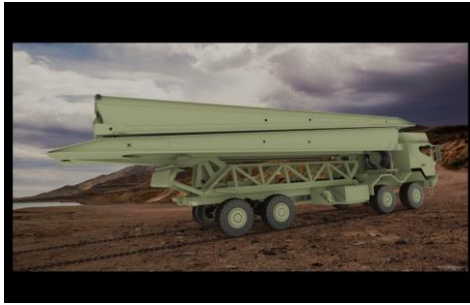
Fig 3.1: The MLC 80+ classification ANACONDA can support the latest and heaviest variants of the LEOPARD 2, M1A2 ABRAMS and CHALLENGER 2
