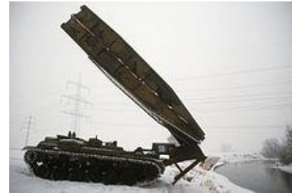
Fig 2.1: REFORGER 1985, an M60 AVLB deploying its bridge on the banks of Lahn River
